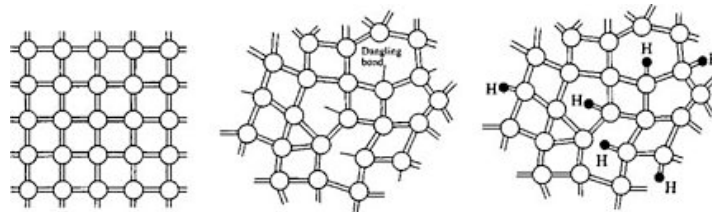
Figure 6.18: Crystalline structure of Si (left), continuous random network of amorphous Si with dangling bonds (centre), hydrogenated amorphous Si (right).
