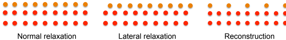
Figure 2.13: Schematic examples of relaxation and reconstruction of a crystal surface.
