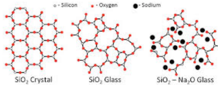
Figure 6.17: Crystalline structure of SiO 2 (left), continuous random network of SiO 2 glass (centre), modified random network of SiO 2 -Na 2 O glass (right).
